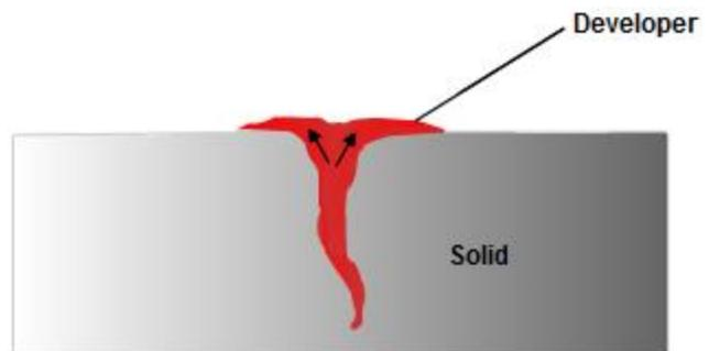
7. Inspection: Inspection is then performed under appropriate lighting to detect indications from any flaws which may be present.
