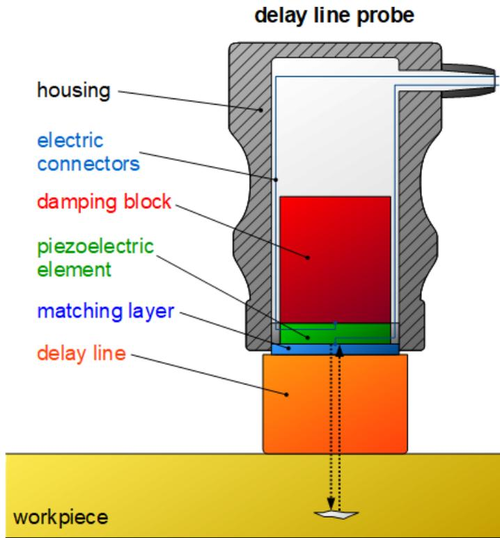
Figure: Components of a delay line probe
