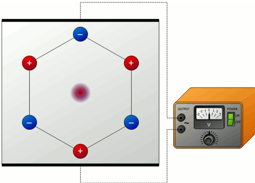
Animation: Piezoelectric crystal on an alternating voltage
