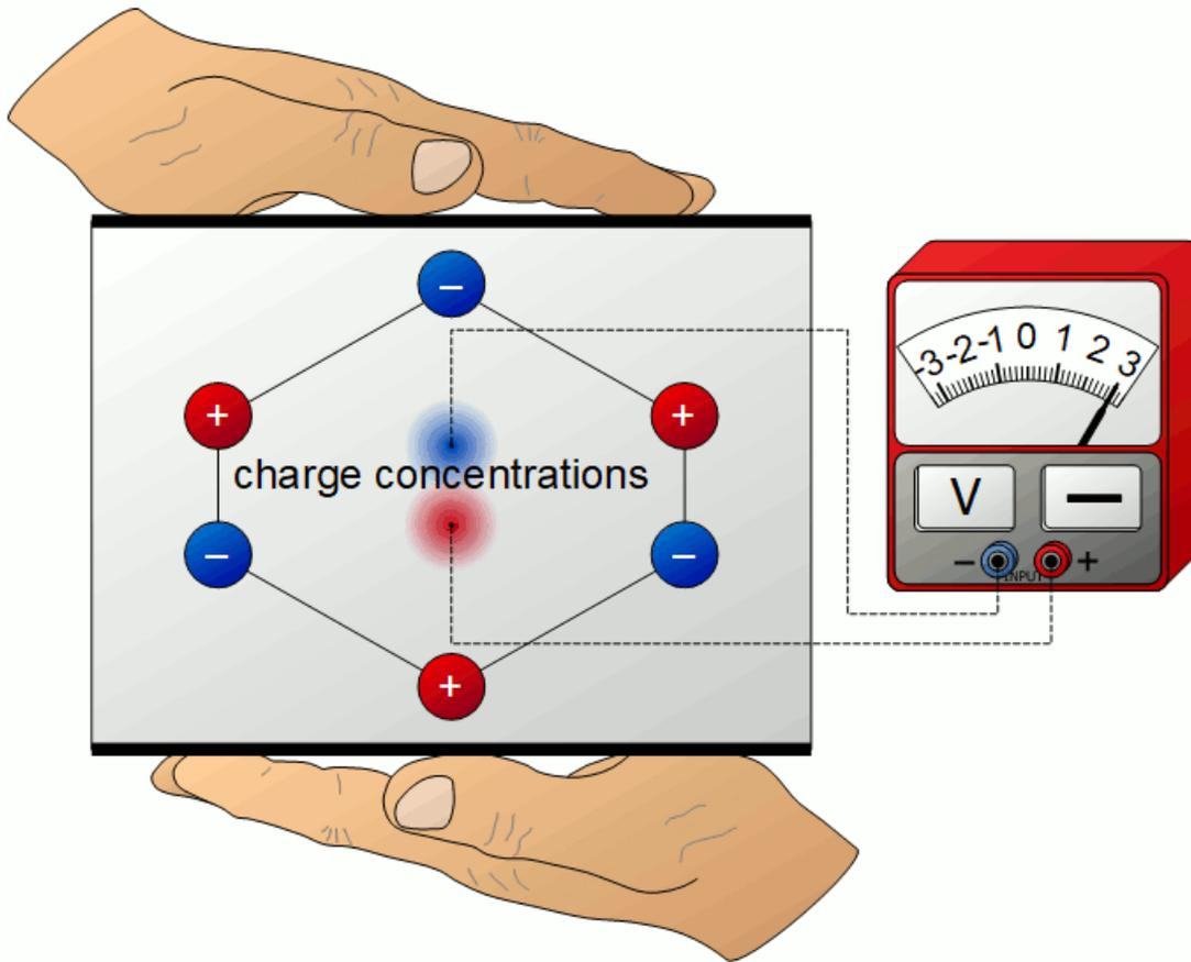
Figure: Piezoelectric effect
