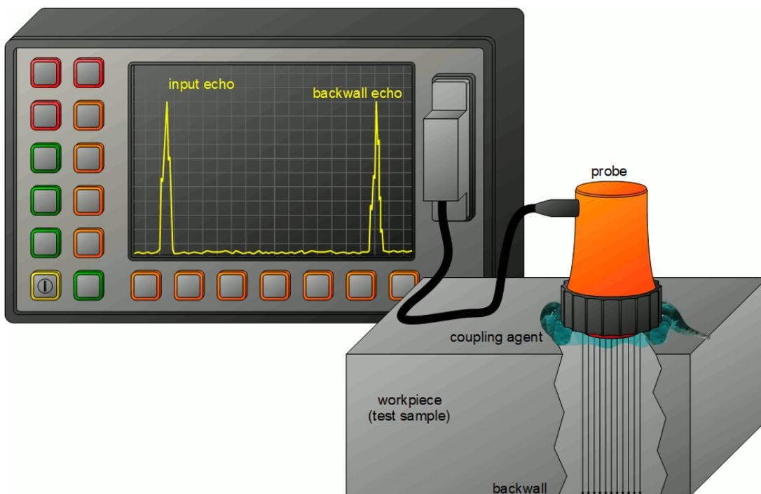
Figure: Principle of ultrasonic testing
