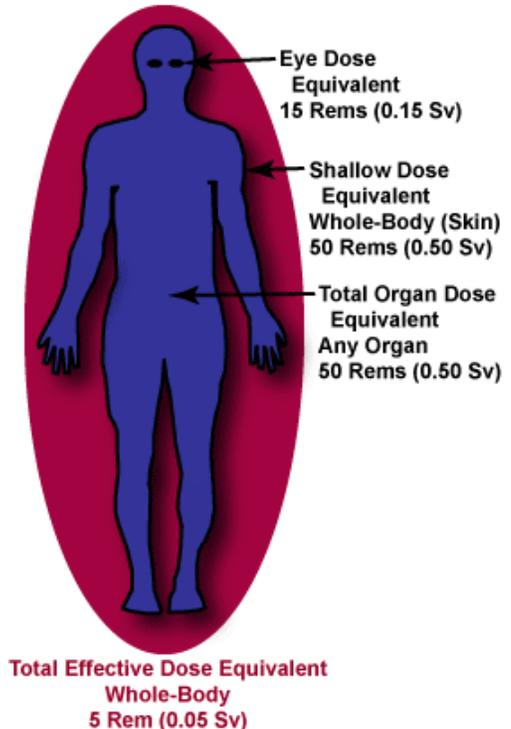
The shallow-dose equivalent is the external dose to the skin of the whole-body or extremities from an external source of ionizing radiation. This value is the dose equivalent at a tissue depth of  $0.007\text{ cm}$  averaged over an area of  $10\text{ cm}^2$ .
