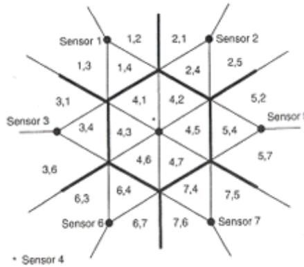
When additional sensors are applied, arrival times and amplitudes help pinpoint the source zone. The ordered pair in lower right figure represents the two sensors detecting the signal in the zone and the order of signal arrival at each sensor. When relating signal strength to peak amplitude, the largest peak amplitude is assumed to come from the nearest sensor, second largest from the next closest sensor and so forth.
