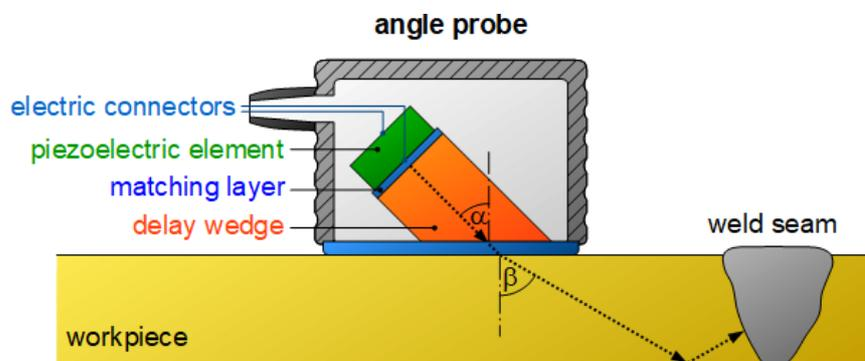
Figure: Components of an angle probe
