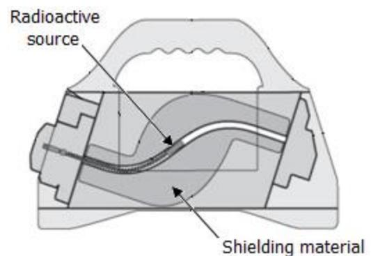
To make a radiographic exposure, a crank-out mechanism and a guide tube are attached to opposite ends of the exposure device. The guide tube often has a collimator (*usually made of tungsten*) at the end to shield the radiation except in the direction necessary to make the exposure.
