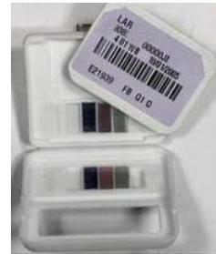
The major advantages of a film badge as a personnel monitoring device are that it provides a permanent record, it is able to distinguish between different energies of photons, and it can measure doses due to different types of radiation. It is quite accurate for exposures greater than 100 *mR*. The major disadvantages are that it must be developed and read by a processor (*which is time consuming*) and prolonged heat exposure can affect the film.
