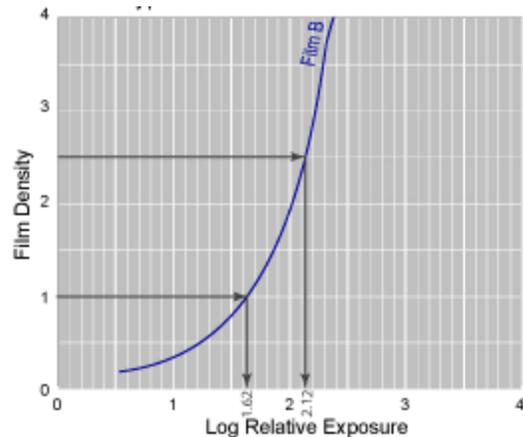
**Example 2:** *Adjusting the Exposure to Allow Use of a Different Film Type*
