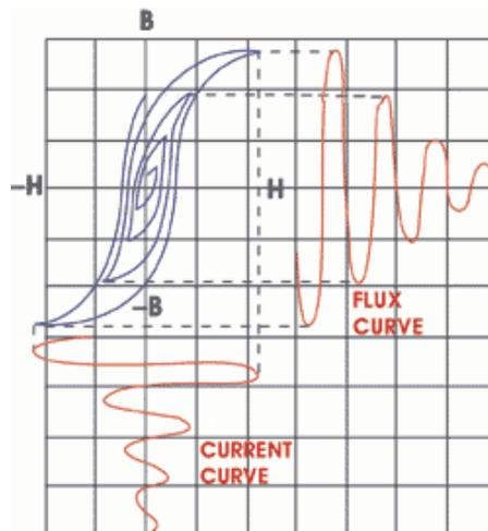
A field meter is often used to verify that the residual flux has been removed from a component. Industry standards usually require that the magnetic flux be reduced to less than 3 Gauss ( $3 \times 10^{-4}$  Tesla) after completing a magnetic particle inspection.
